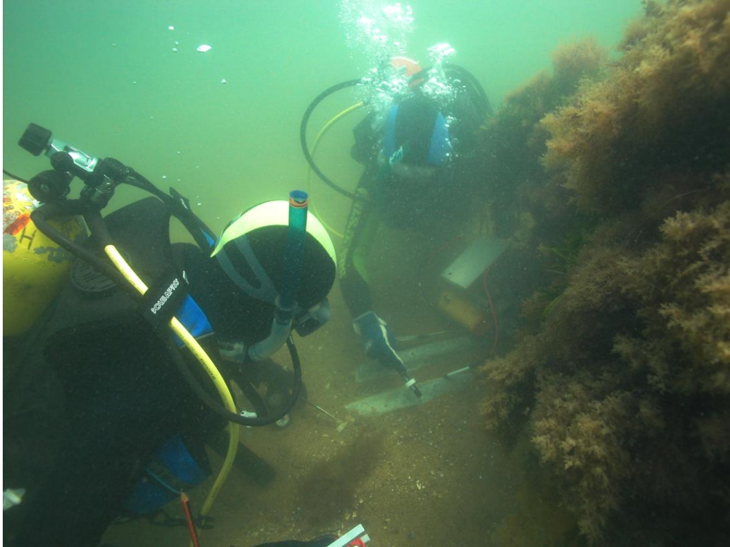
Figure 2. Divers measuring corrosion potentials on anodes treating gun barrels in-situ from HMVS Cerberus in 2009 (photo courtesy of Heritage Victoria S117).
